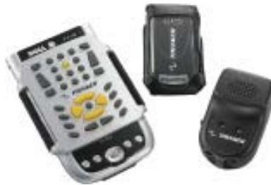
Figure 2 HumanWare Trekker accessible GPS with hardware component. Maestro tools do not have to be activated/used.
