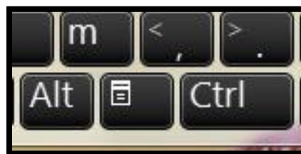
Figure 3 Image of AppKey between the Alt and Ctrl keys on the main keyboard area.
